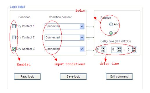
These are the settings for devices controlled by dry contact after the input conditions valid.
